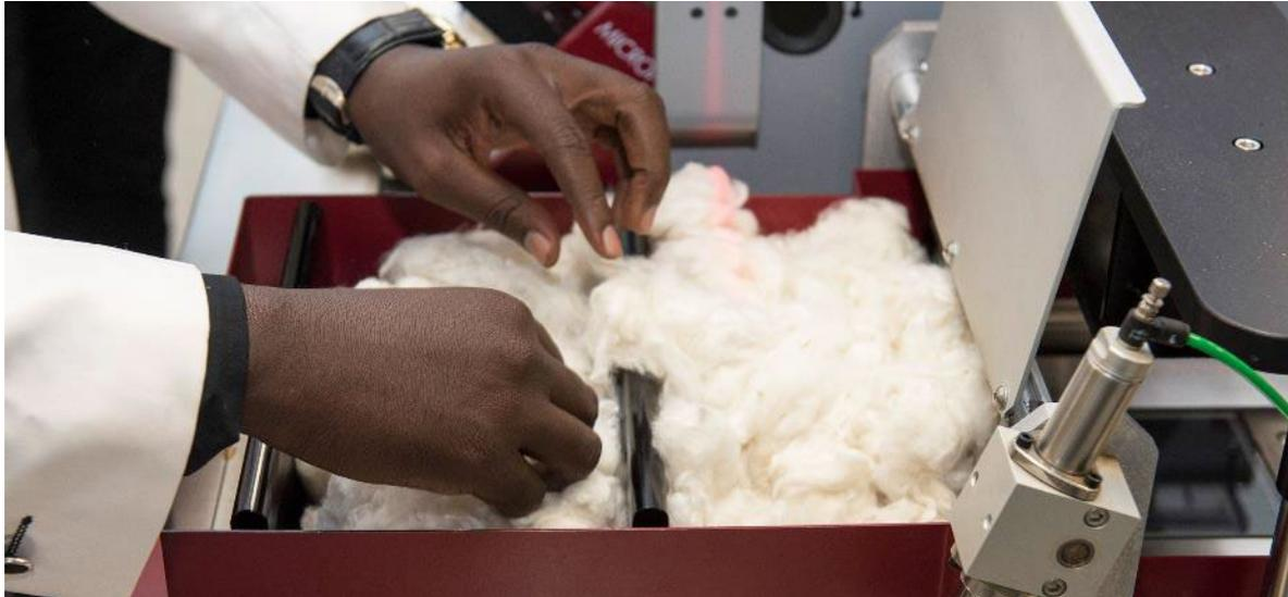
Cotton quality testing with an HVI © Bremen Cotton Exchange
